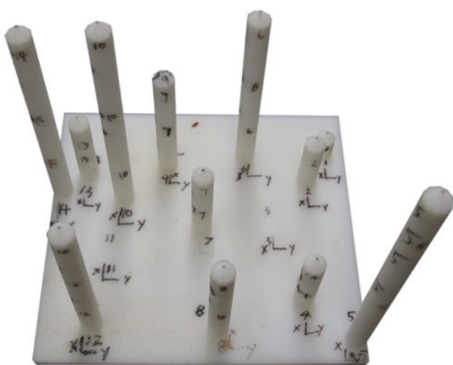
Fig. 2. Calibration rig used for defining the spatial coordinates in the glass tanks for analysis with the Direct Linear Transformation (DLT) algorithm
